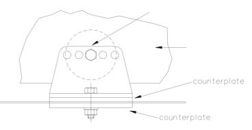
There is also an option within FIA Appendix J regulations for mounting seats to a transverse cross member; the drawing below (reproduced from FIA Appendix J) details the requirements for this mounting method. The transverse cross member of either square or tube section with end plates is bolted to a counter plate at each end; the counter plate is welded to the transmission tunnel and the bodyshell outer rails.
